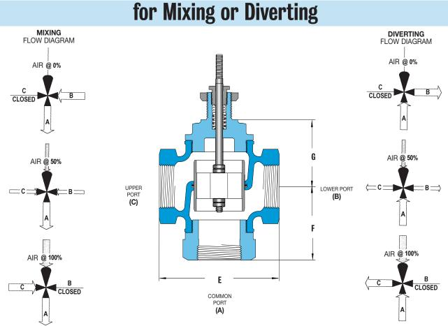
Trerice 3-Way Valves are not designed for use in steam applications. To properly control the mixing of two flows, inlet pressures at ports B and C should be as equal as possible.
