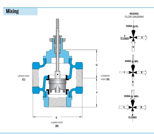
Trerice 3-Way Valves are not designed for use in steam applications.
