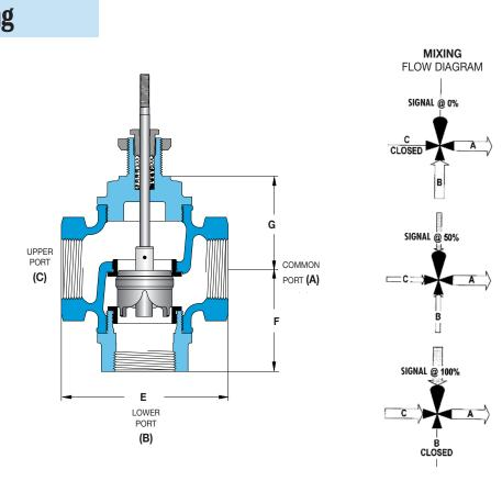
Trerice 3-Way Valves are not designed for use in steam applications. To properly control the mixing of two flows, inlet pressures at ports B and C should be as equal as possible.
